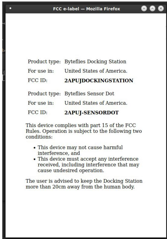
It should be noted that the Sensor Dot can't be turned on without first using the Docking Station, and the user will this always have seen this message.
