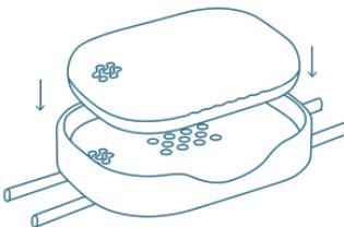
**Step 6.** You can record for up to 24 hours on a single charge. To complete a recording, lift the **Sensor Dot** out of the **4-Wire Cradle** and place it back in a free slot on the **Docking Station**. Its LED should turn orange to indicate data transfer has started.
