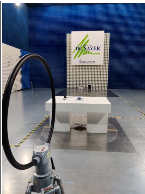
Spurious emission set-up (0.09-30MHz) 3m
