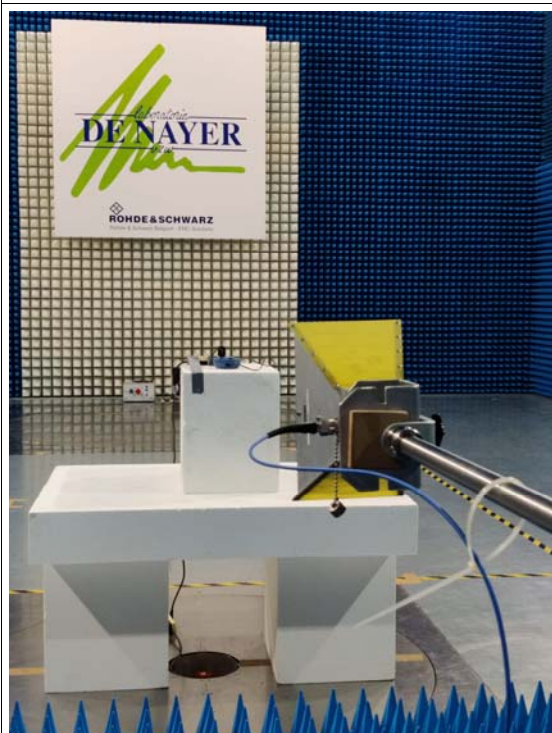
Spurious emission set-up (1-18GHz) 3m
