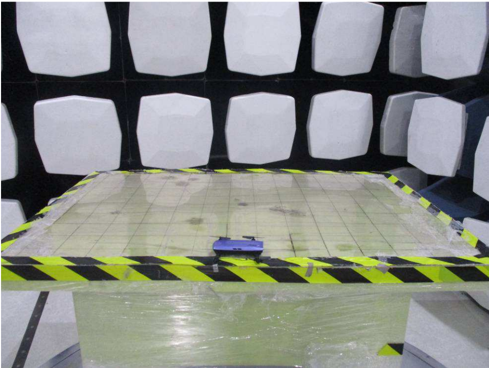
Up to 1G (EUT was placed in the centre of the turntable)
