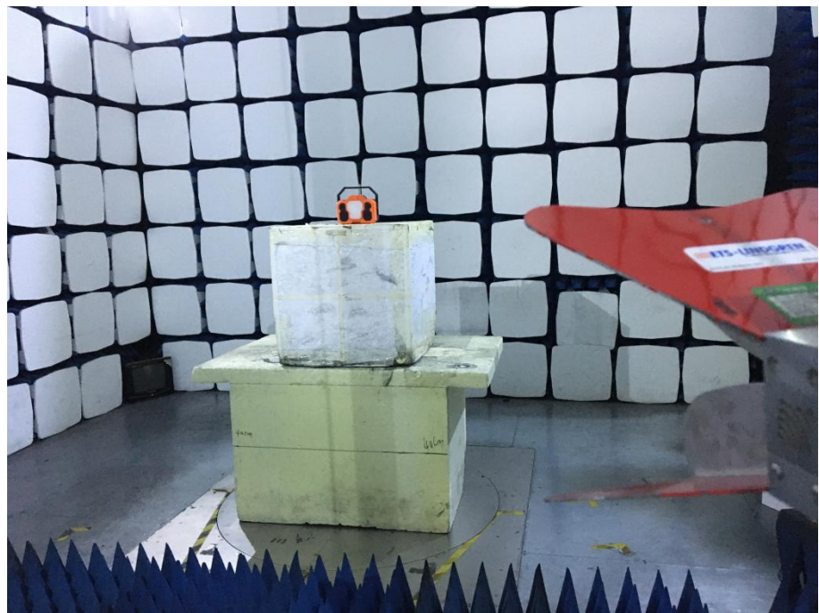
Radiation Emission Test Setup (1GHz to 18GHz)
