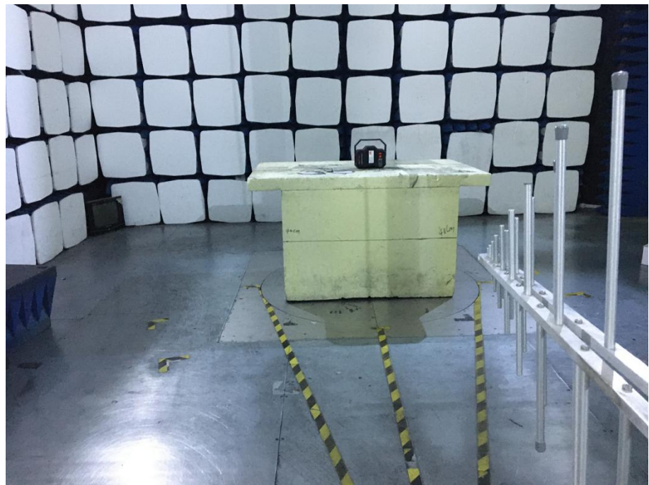
Radiation Emission Test Setup (30MHz to 1GHz)
