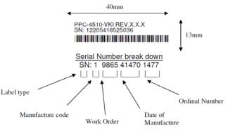
a. Label type - SN for Serial Number type, final assembly.
