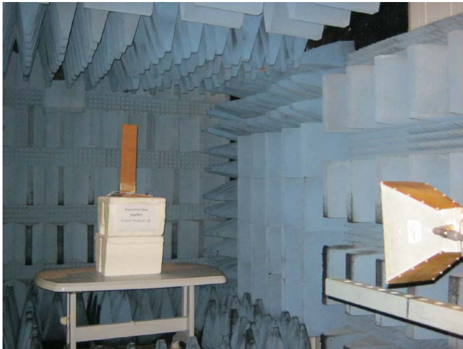
Figure 6. Radiated Emission Test, 1-18GHz
