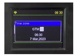
At that time, rotate  $[\checkmark 100]$  to select time zone in GTM:-12.0, -11.0, -10.0, -9.0, -8.0, -7.0, -6.0, -5.0, -4.0, -3.0, -2.0, -1.0, +0, +1.0, +2.0, +3.0, +4.0, +5.0, +6.0, +7.0, +8.0, +9.0, +10.0, +11.0, +12.0. After the time zone is selected, light press [ENTER] to confirm it.  $\approx$ : The date displayed will be automatically updated after network is successfully connected.
