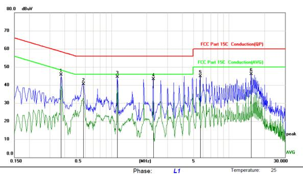
Limit: FCC Part 15C Conduction(QP)
