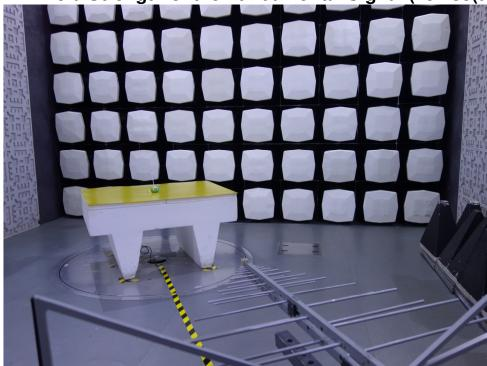
1.2 Radiated Emissions (30MHz-1GHz) Test Setup
