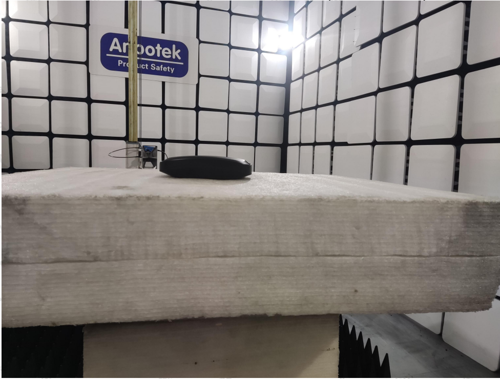
Photo of Radiation Emission Test (above 1GHz)
