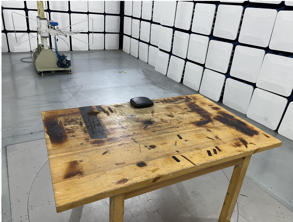
Photo of Radiation Emission Test (below 1GHz)
