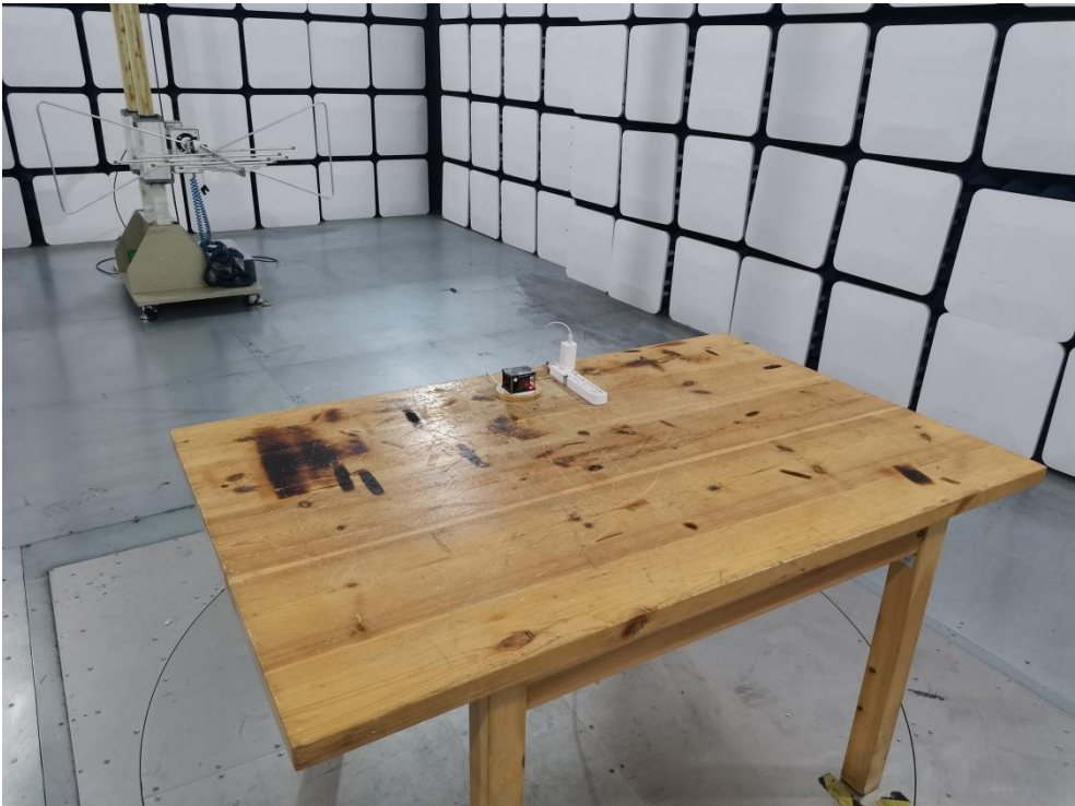
Photo of Radiation Emission Test
