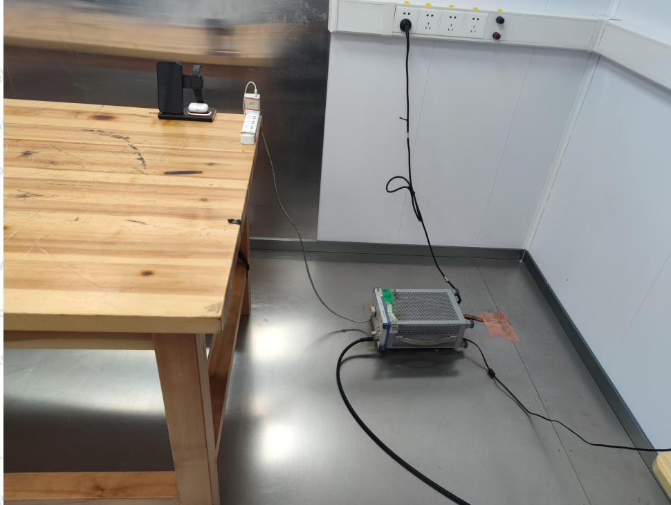
Photo of Conducted Emission Measurement
