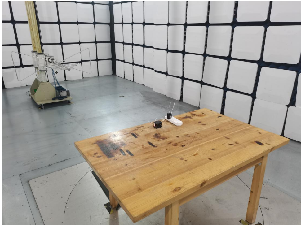
Photo of Radiation Emission Test
