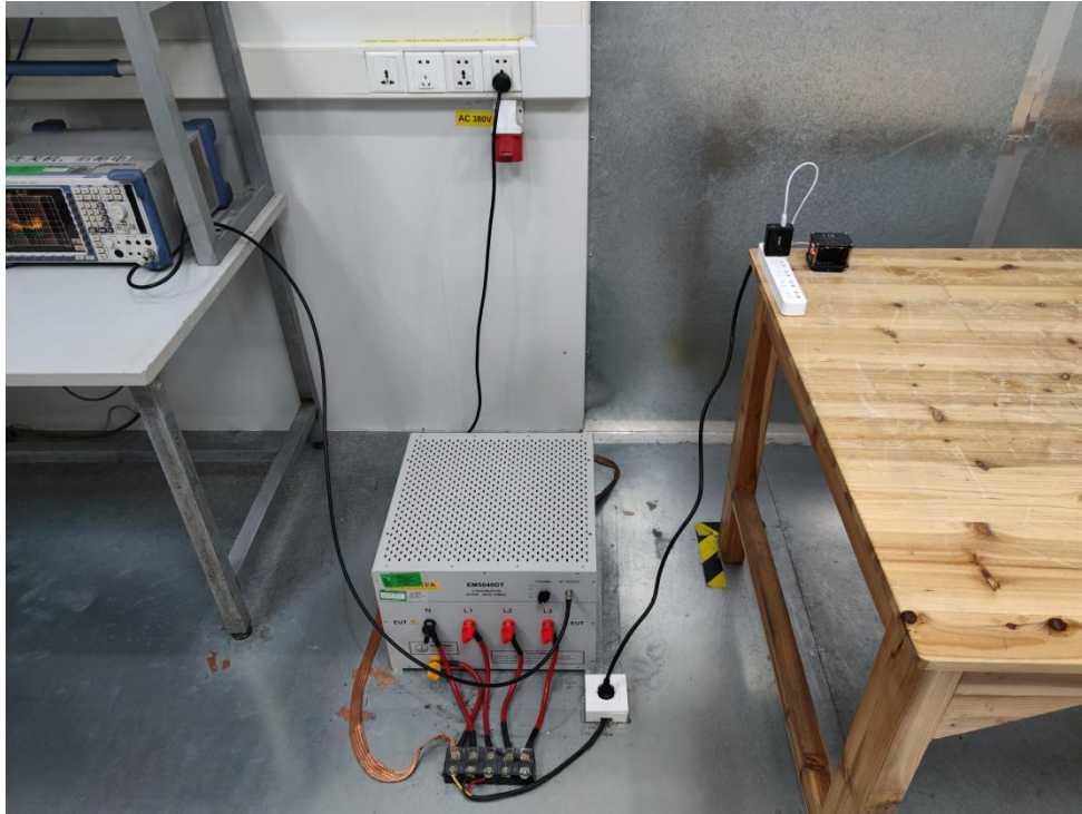
Photo of Conducted Emission Measurement
