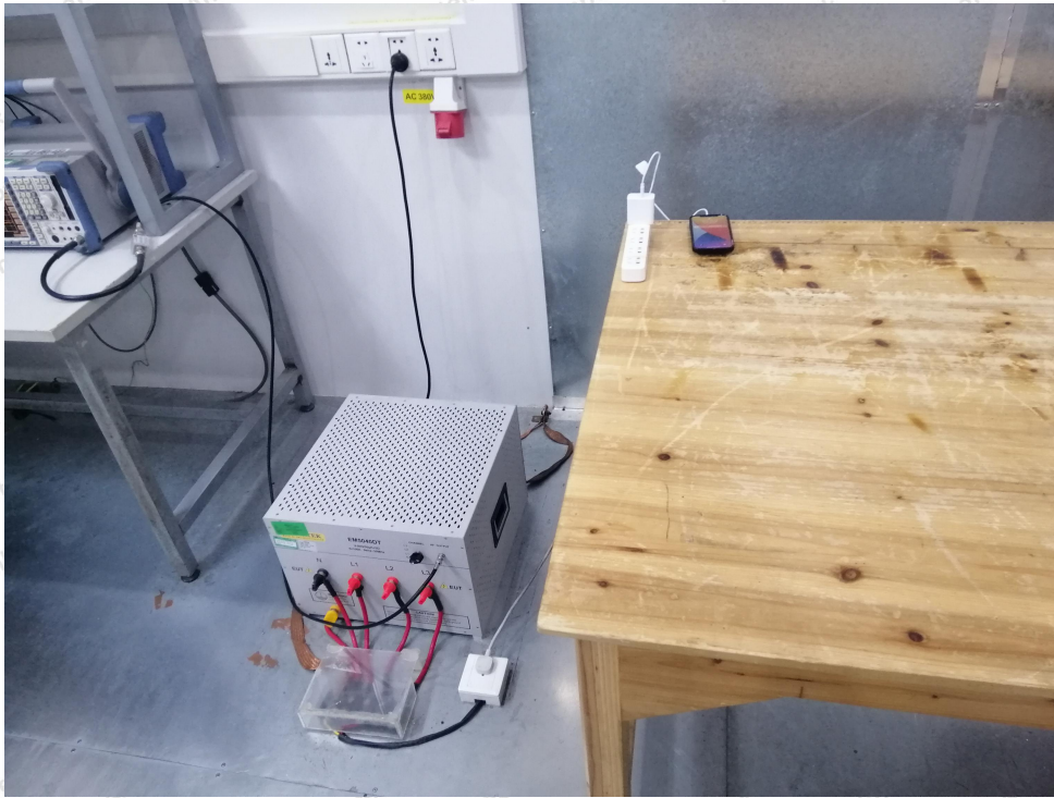
Photo of Conducted Emission Measurement
