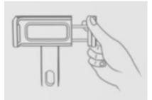
4. Clip the smartphone into the holder. Place the smartphone on the center of the wireless charger or adjust the placement position until the charging process starts. The red led indicator goes out and blue led indicator lights up.
