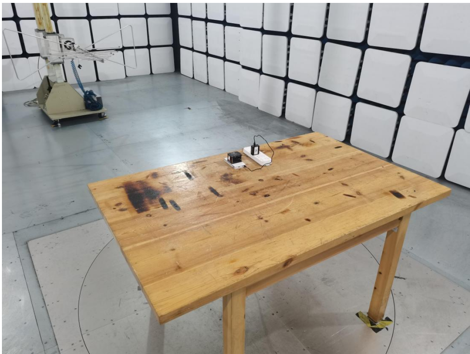
Photo of Radiation Emission Test
