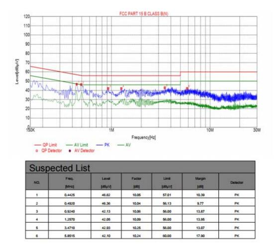
Remark: Margin = Limit – Level Level=Test receiver reading + factor Factor= Antenna factor + cable loss- Amp factor
