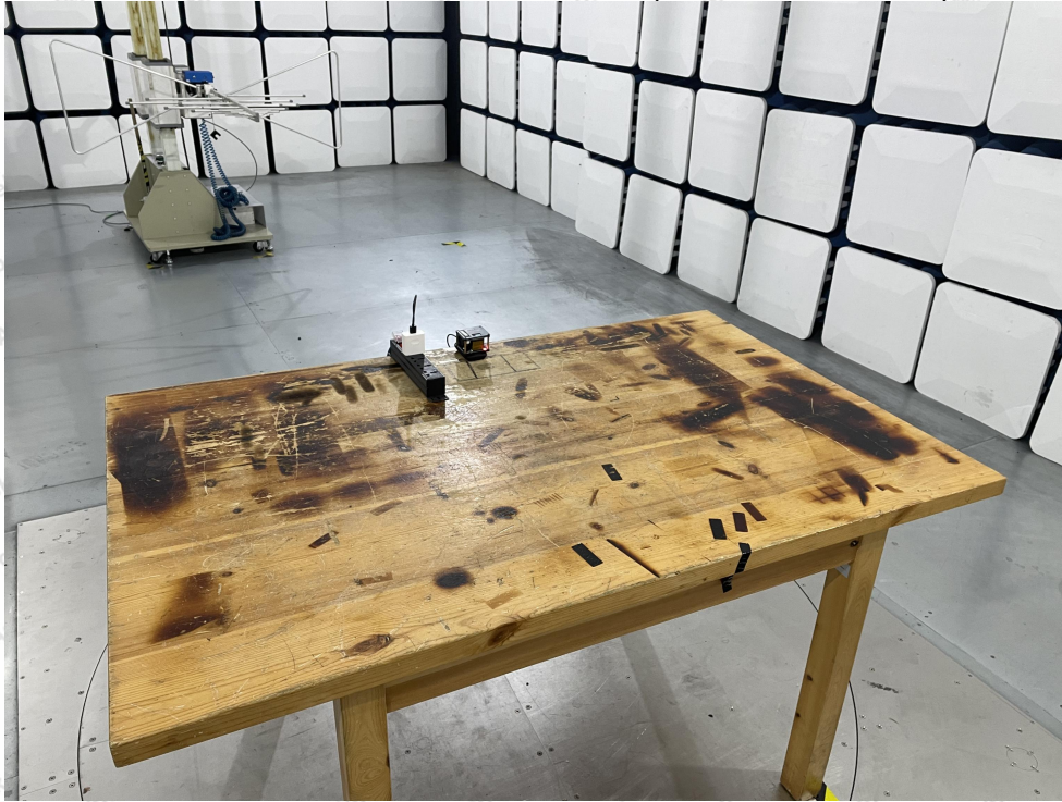
Photo of Radiation Emission Test (30MHz~1000MHz)
