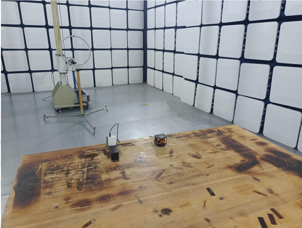
Photo of Radiation Emission Test (below 30MHz)
