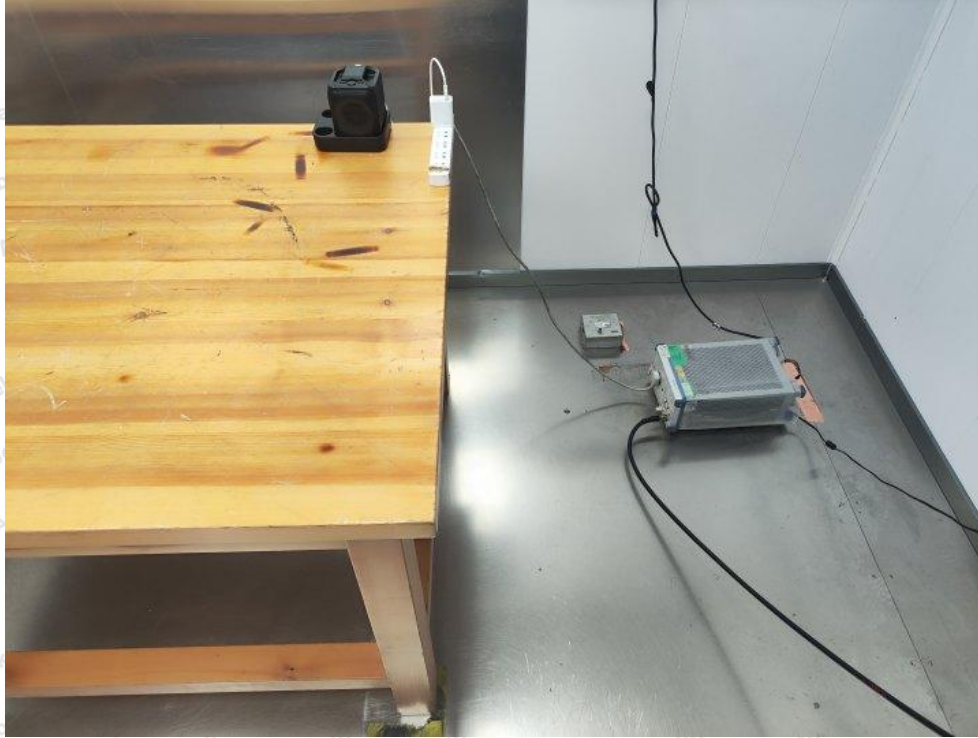
Photo of Radiation Emission Test (below 1GHz)
