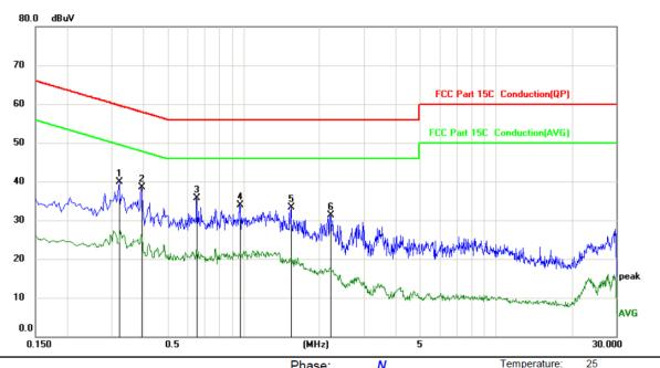
Limit: FCC Part 15C Conduction(QP)
