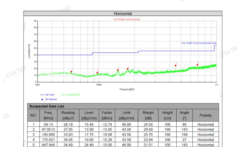
Note:1).Level (dBµV/m)= Reading (dBµV)+ Factor (dB/m)
