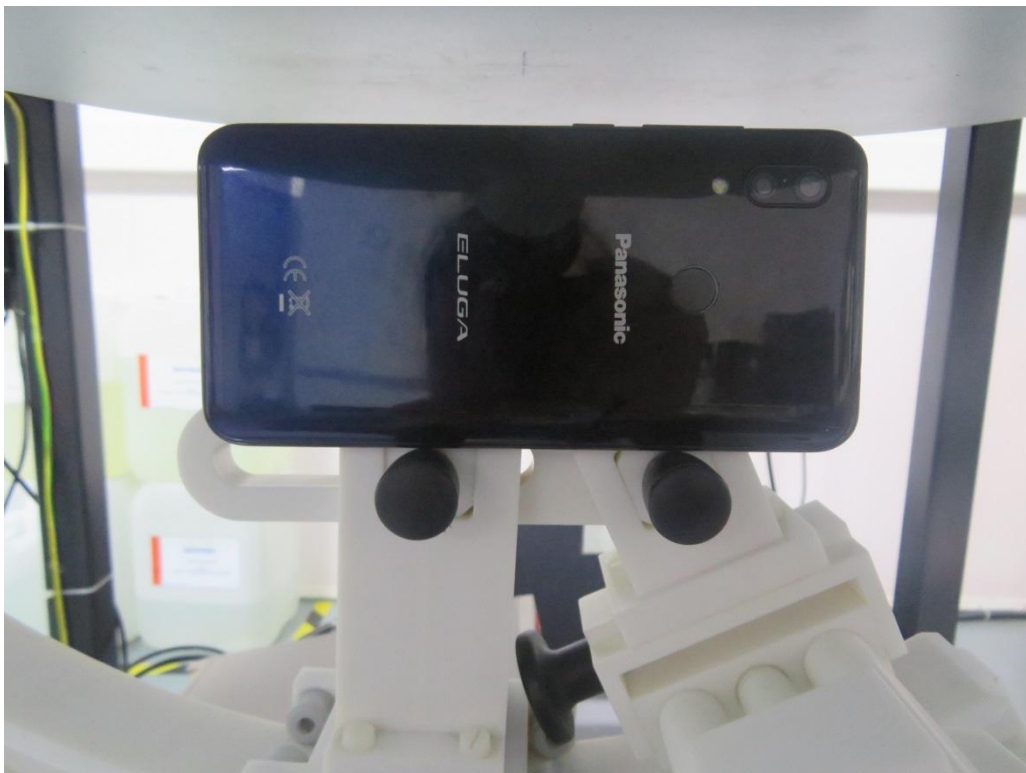
10mm body-worn Right Side Setup Photo (hotspot)
