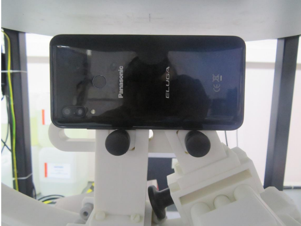
10mm body-worn Left Side Setup Photo (hotspot)
