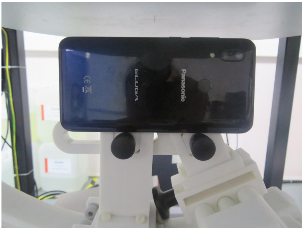
10mm body-worn Right Side Setup Photo (hotspot)
