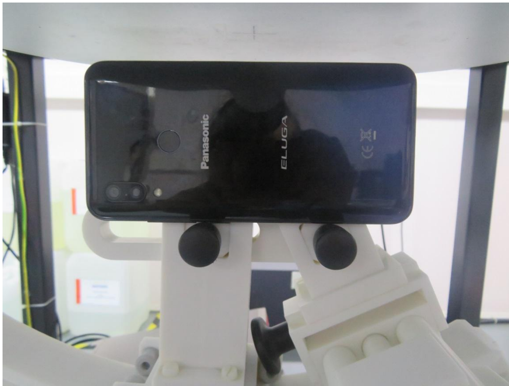
10mm body-worn Left Side Setup Photo (hotspot)
