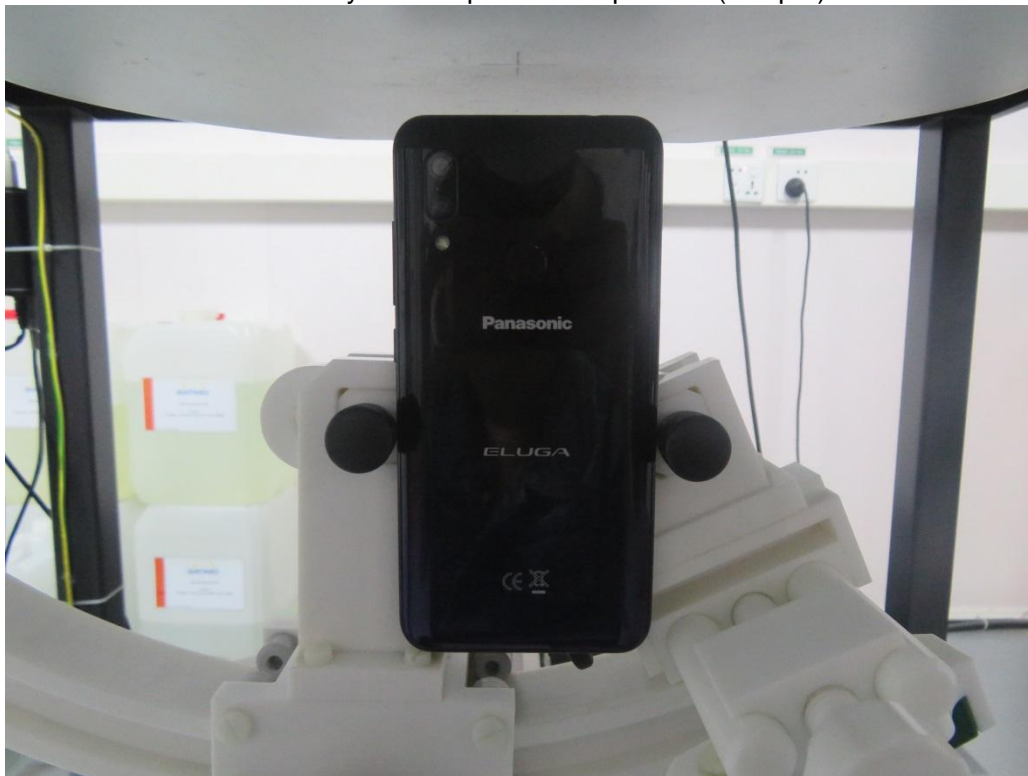
10mm body-worn Top Side Setup Photo (hotspot)
