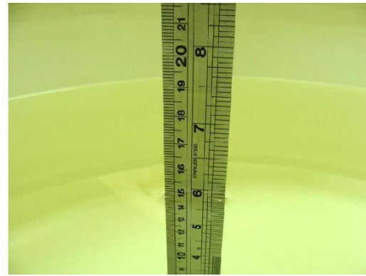
Fig 7.2 Photo of Liquid Height for Body SAR
