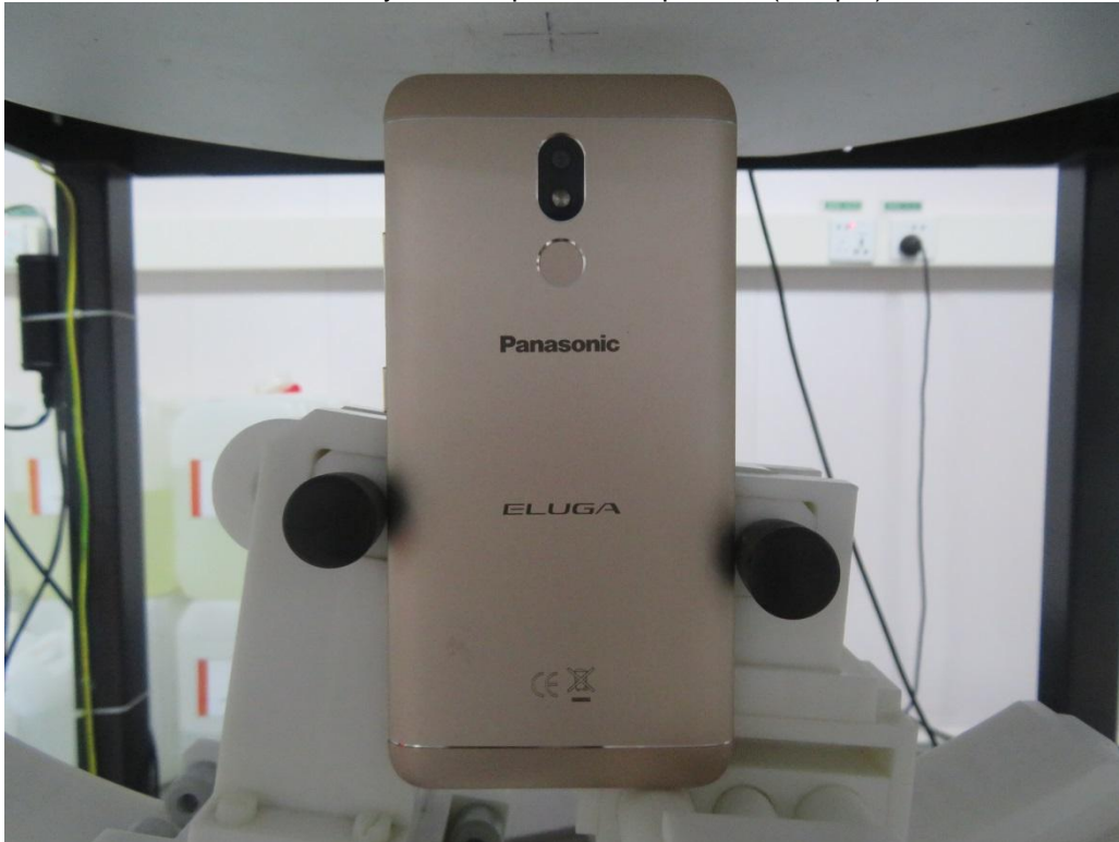
10mm body-worn Top Side Setup Photo (hotspot)
