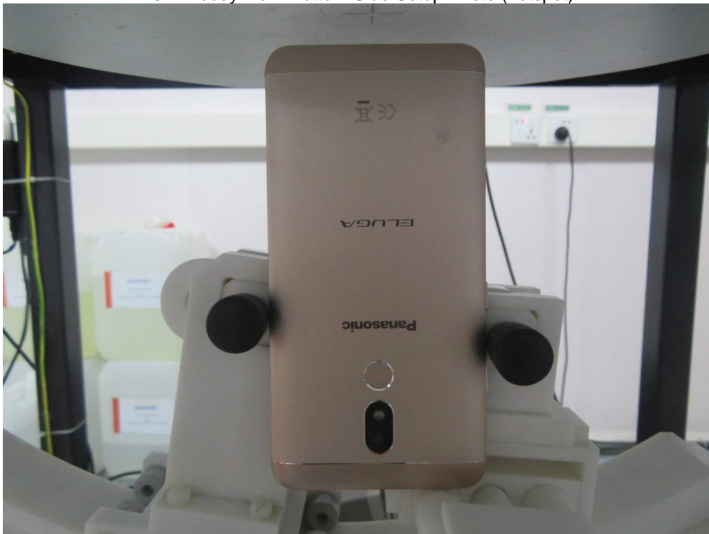
10mm body-worn Bottom Side Setup Photo (hotspot)
