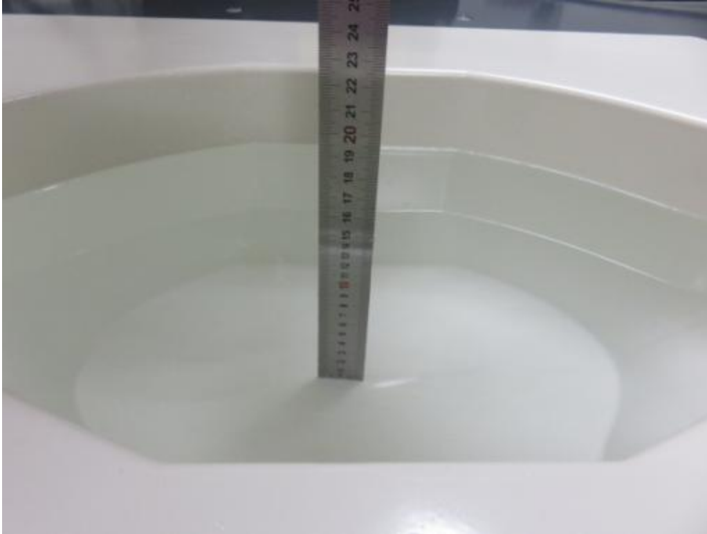
Photograph of the depth in the Body Phantom (750MHz, 15.4cm depth)
