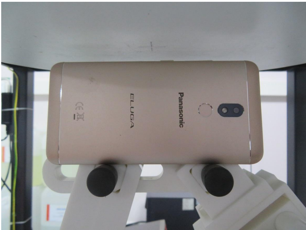
10mm body-worn Right Side Setup Photo (hotspot)
