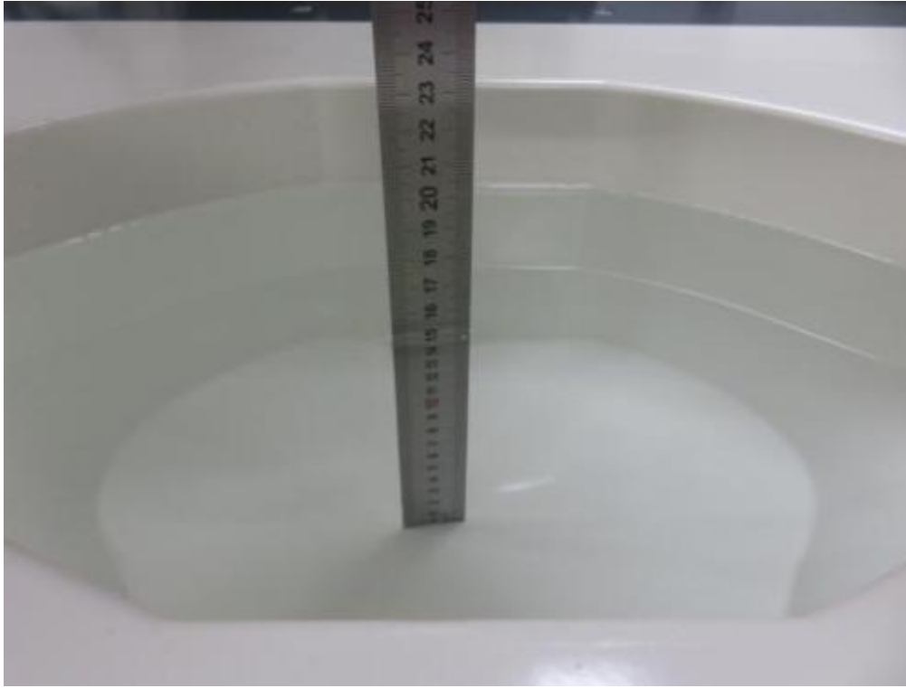
Photograph of the depth in the Body Phantom (2450MHz, 15.3cm depth)
