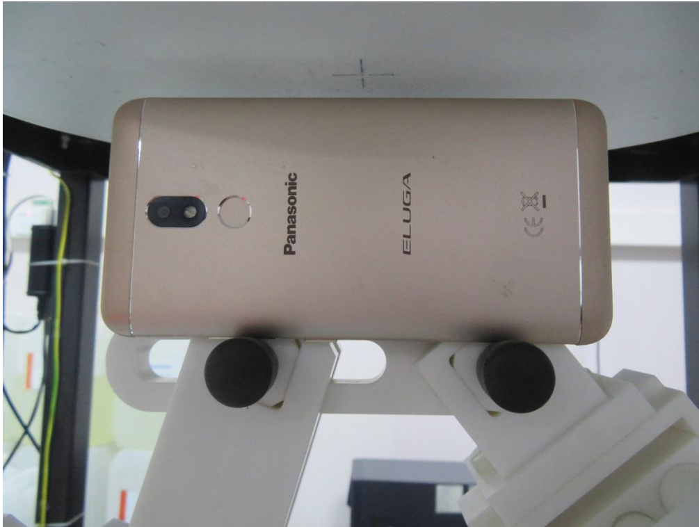
10mm body-worn Left Side Setup Photo (hotspot)
