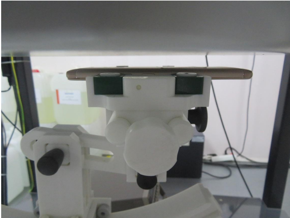
10mm body-worn Back Side Setup Photo (hotspot)
