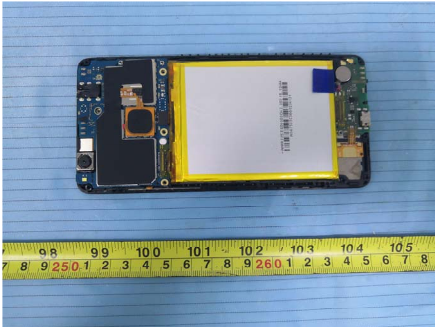
EUT – Cover off View 3
