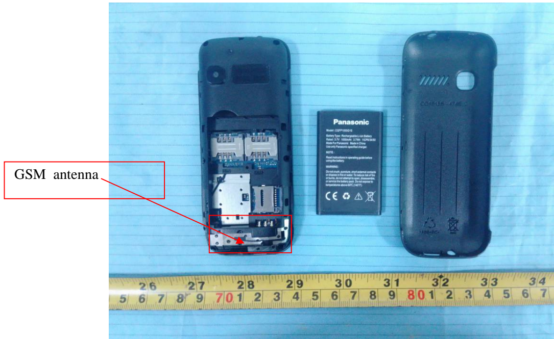
EUT – Cover off View 1
