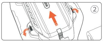
Open the two locks on the left and right respectively, push back to remove the battery pack.
