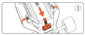
Lift the battery connector and push the battery in. Connect the power connector and make sure both locks are well fasten.
