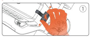
Press the buckle to unplug the power connector.
