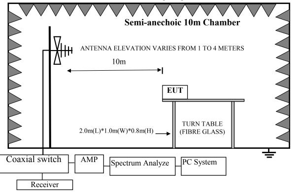
4.2.2.In 10m Anechoic Chamber Test Setup Diagram for 1-6GHz
