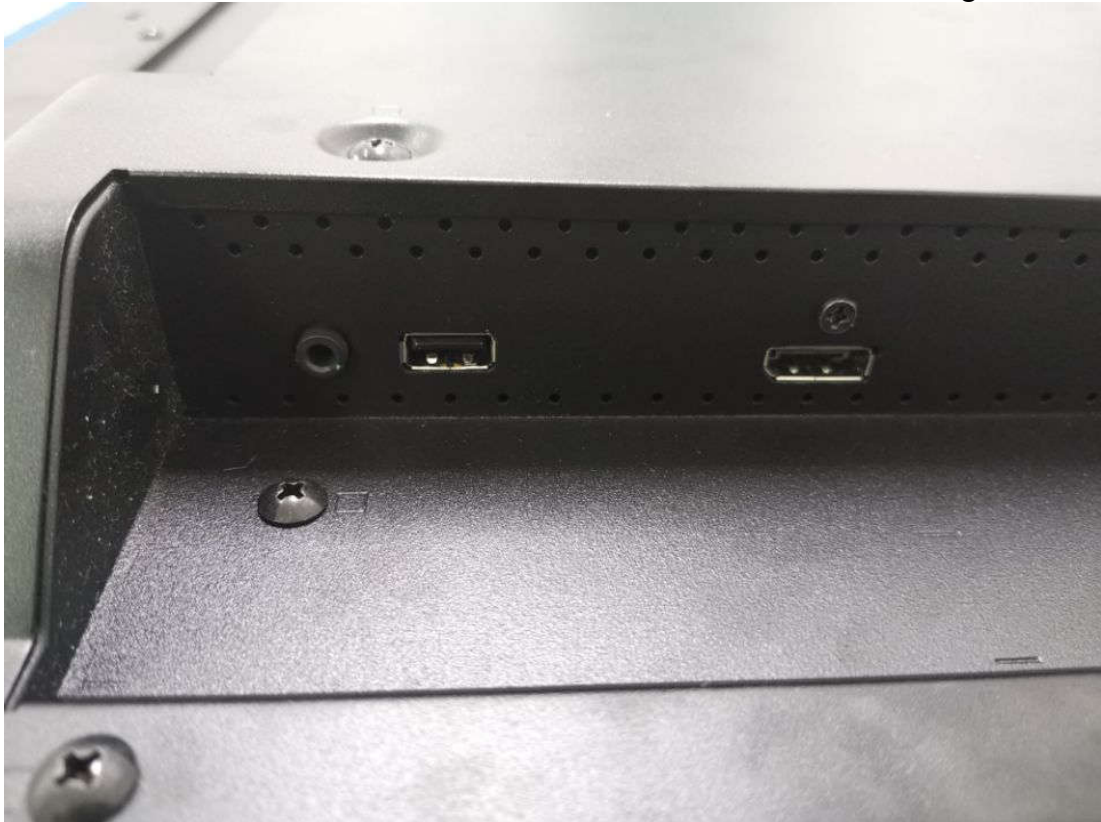
Figure 11 Signal Port of the EUT
