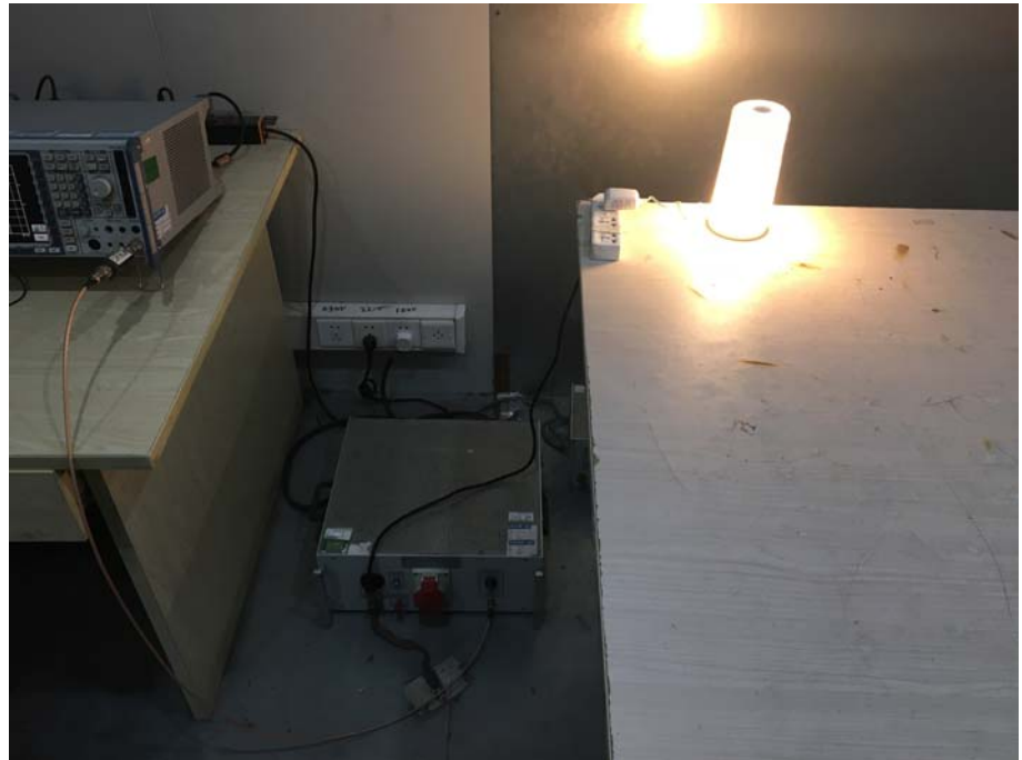
Conducted Emission Test Setup
