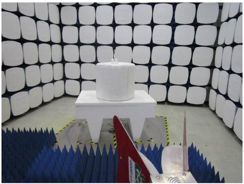
1.2 Radiated Spurious Emissions Test Setup
