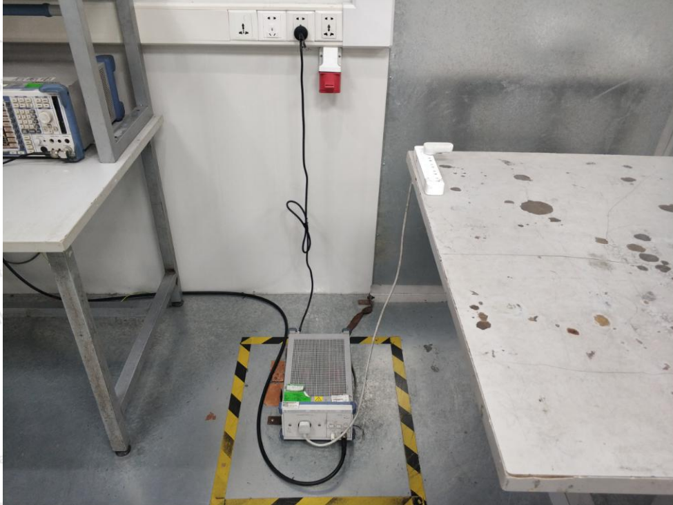
Photo of Conducted Emission Measurement
