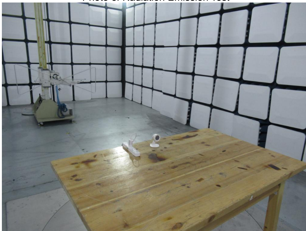
Photo of Radiation Emission Test
