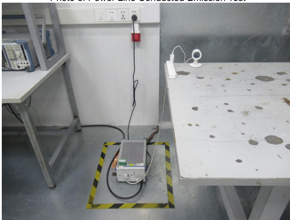
FCC ID: 2APSE-CAMERA Photo of Power Line Conducted Emission Test
