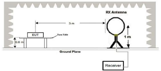
(2) Radiated Emission Test-Up Frequency 30MHz~1GHz
