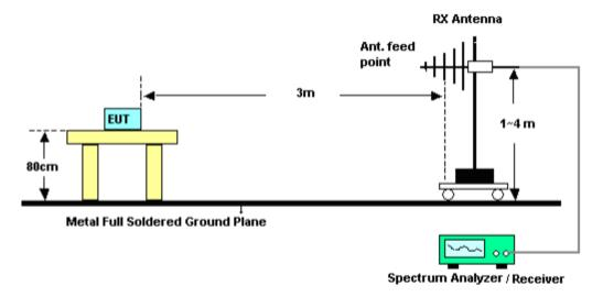
(C) Radiated Emission Test-Up Frequency Above 1GHz
