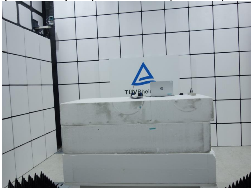
Photograph 2: Test Setup for Spurious Emissions (Front View 2)
