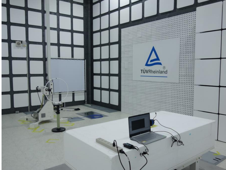
Photograph 6: Test Setup for Spurious Emissions (Back View 4)
