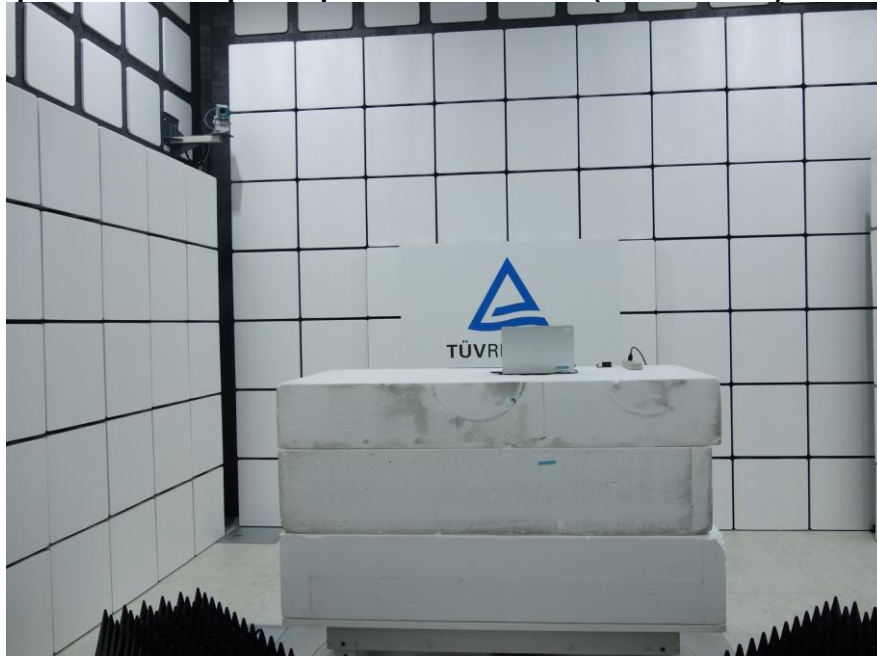
Photograph 2: Test Setup for Spurious Emissions (Front View 2)
