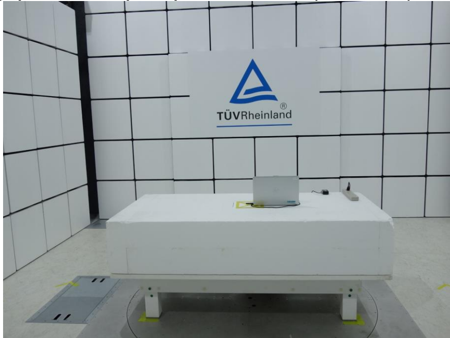
Photograph 1: Test Setup for Spurious Emissions (Front View 1)
