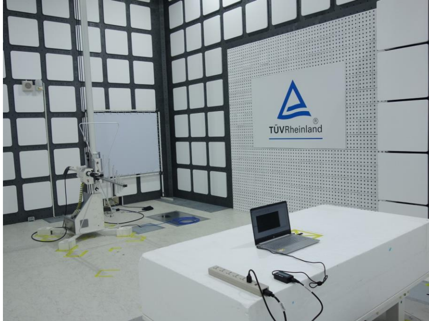
Photograph 3: Test Setup for Spurious Emissions (Back View 1)
