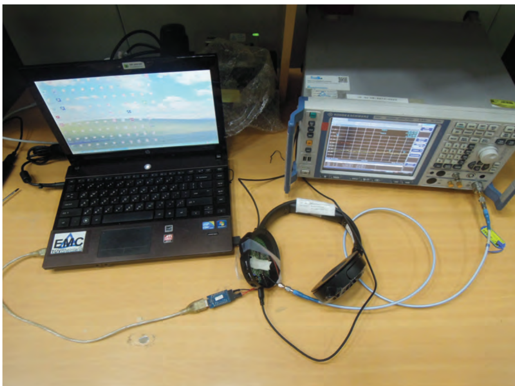
Photograph 4: Set-up for Conducted testing
