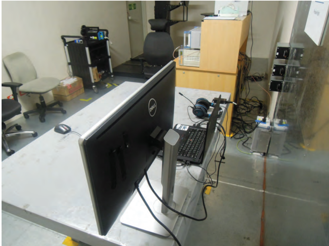
Photograph 6: Set-up for Mains Conducted testing (Front)
