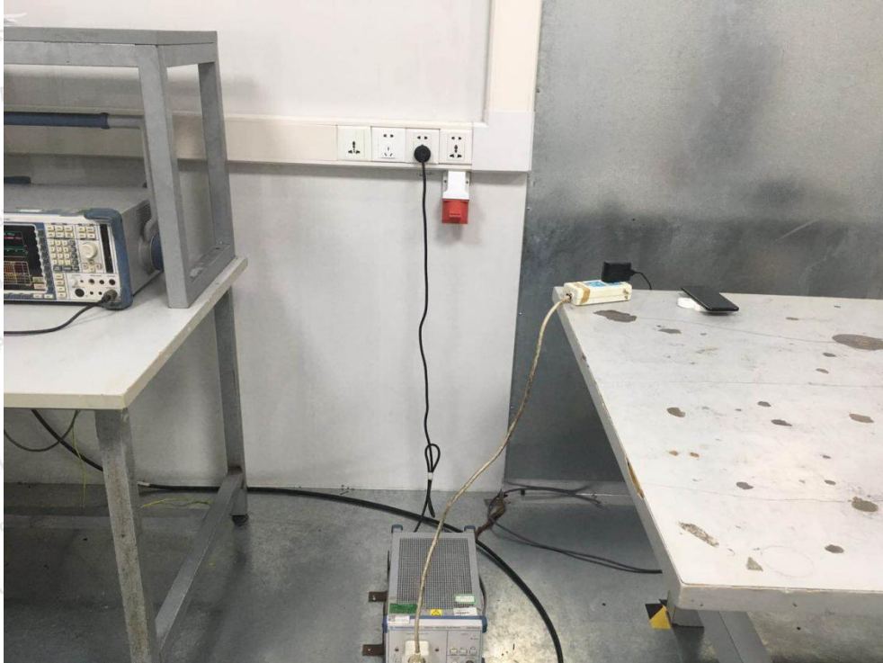
Photo of Conducted Emission Measurement
