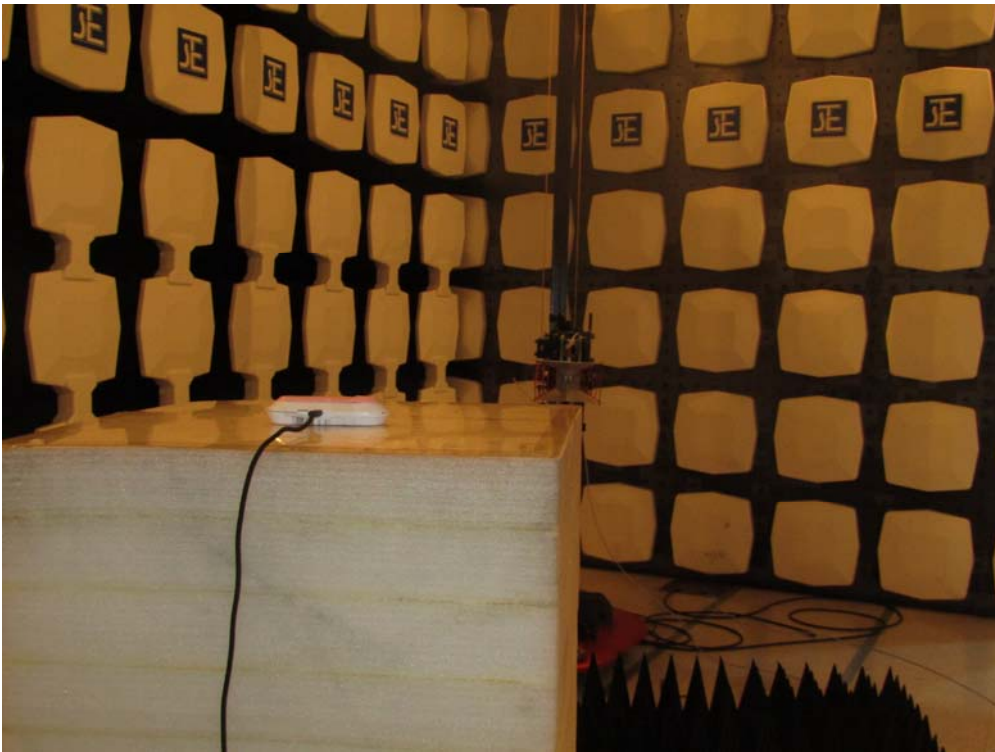
Measurement of Radiated Emission Test Set Up
