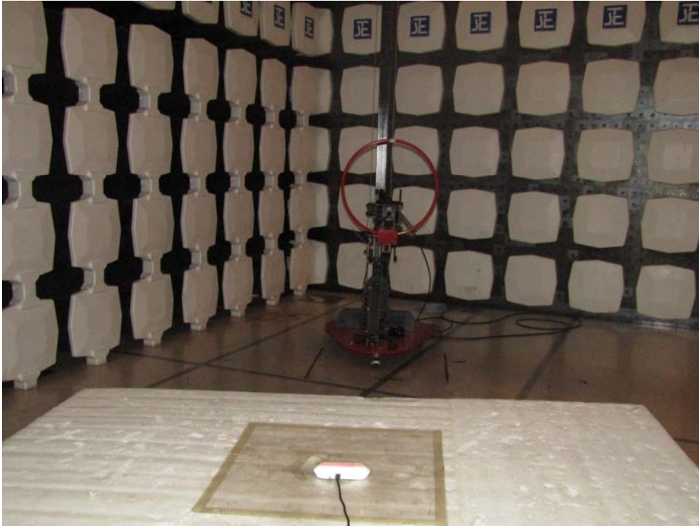
Measurement of Radiated Emission Test Set Up
