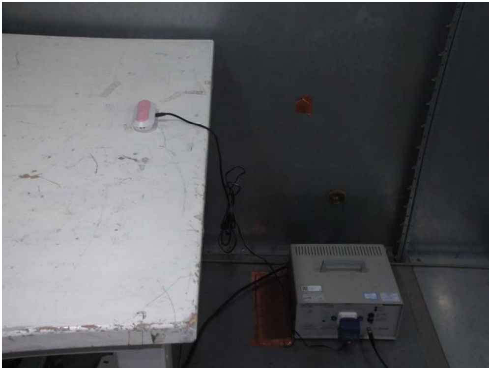
Measurement of Conducted Emission Test Set Up
