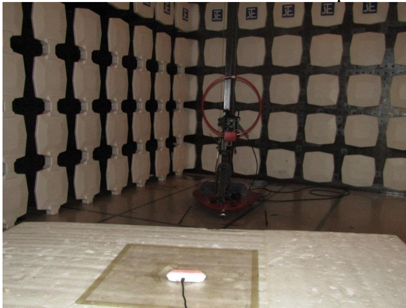
Measurement of Radiated Emission Test Set Up
