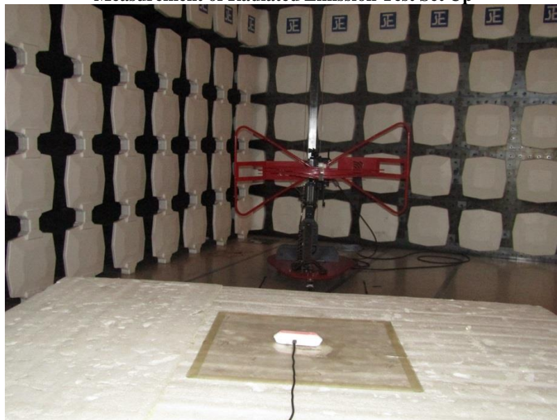
Measurement of Radiated Emission Test Set Up
