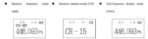
In the power-on state, press the (V/M) key to switch between the above three modes.
