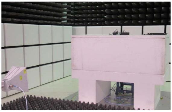
Radiated Emission Set up Photos (Front View)
