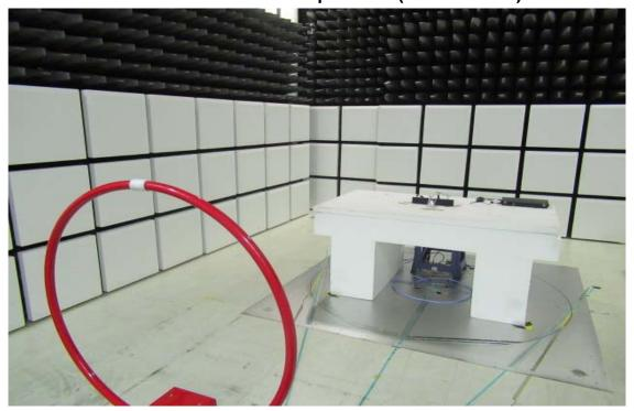
Radiated Emission Set up Photos (Below 1GHz)
