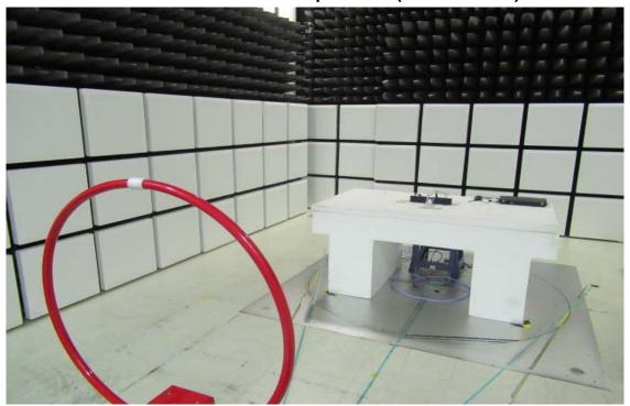
Radiated Emission Set up Photos (Below 1GHz)
