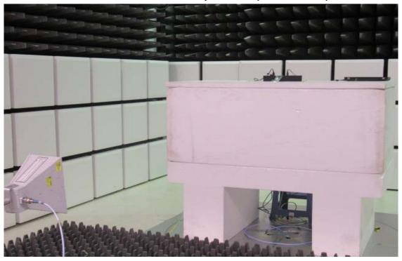
Radiated Emission Set up Photos (Front View)
