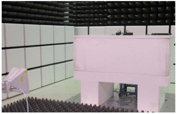
Radiated Emission Set up Photos (Front View)
