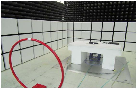
Radiated Emission Set up Photos (Below 1GHz)
