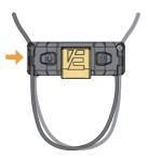
Reattach wire into Chin-Mic wire clip by pressing into the groove.
