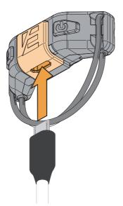
Insert USB charging cable into USB port located on bottom side of the Chin-Mic to charge Slimbuds.
