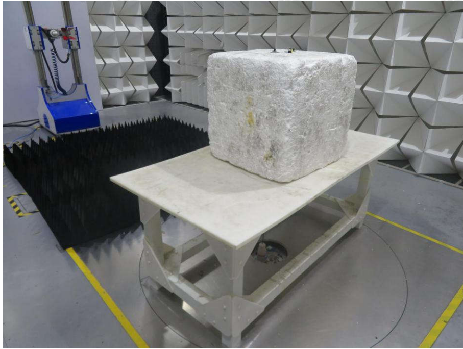
Radiated spurious emission Test Setup-3(Above 1GHz)
