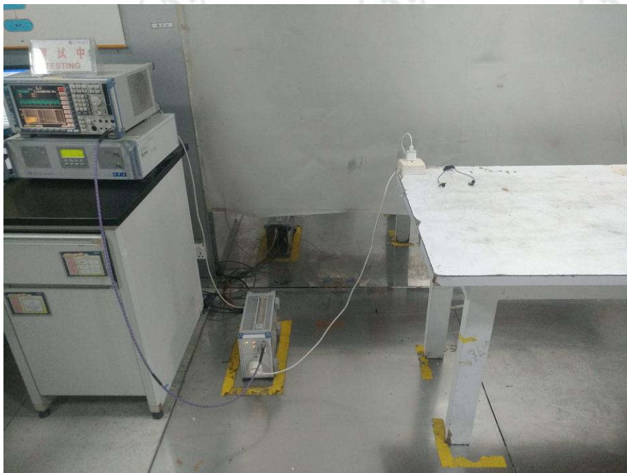
Conducted Emissions Test Setup
