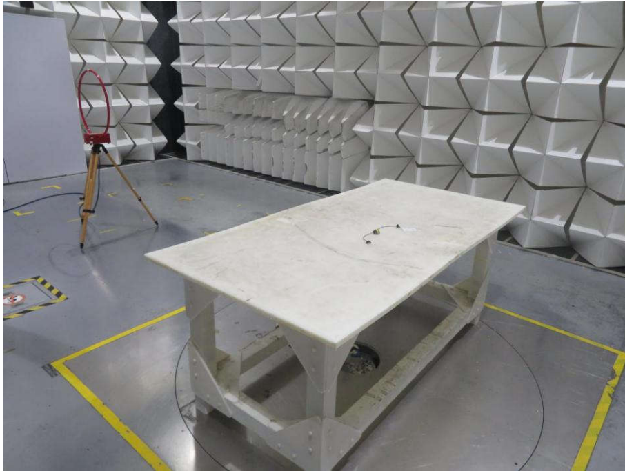
Radiated spurious emission Test Setup-1(Below 30MHz)
