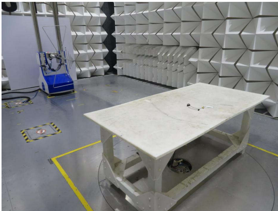
Radiated emission Test Setup-2(30MHz - 1GHz)
