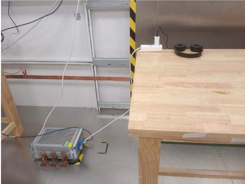
AC Power Line Conducted Emission
